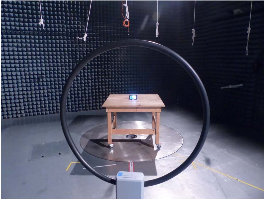
Photo 2: Test setup for radiated measurements (Enclosure, below 30 MHz, intentional radiator §15). The construction visible on the top of the photo consists of non-conductive ropes which do not affect the measurement results.
