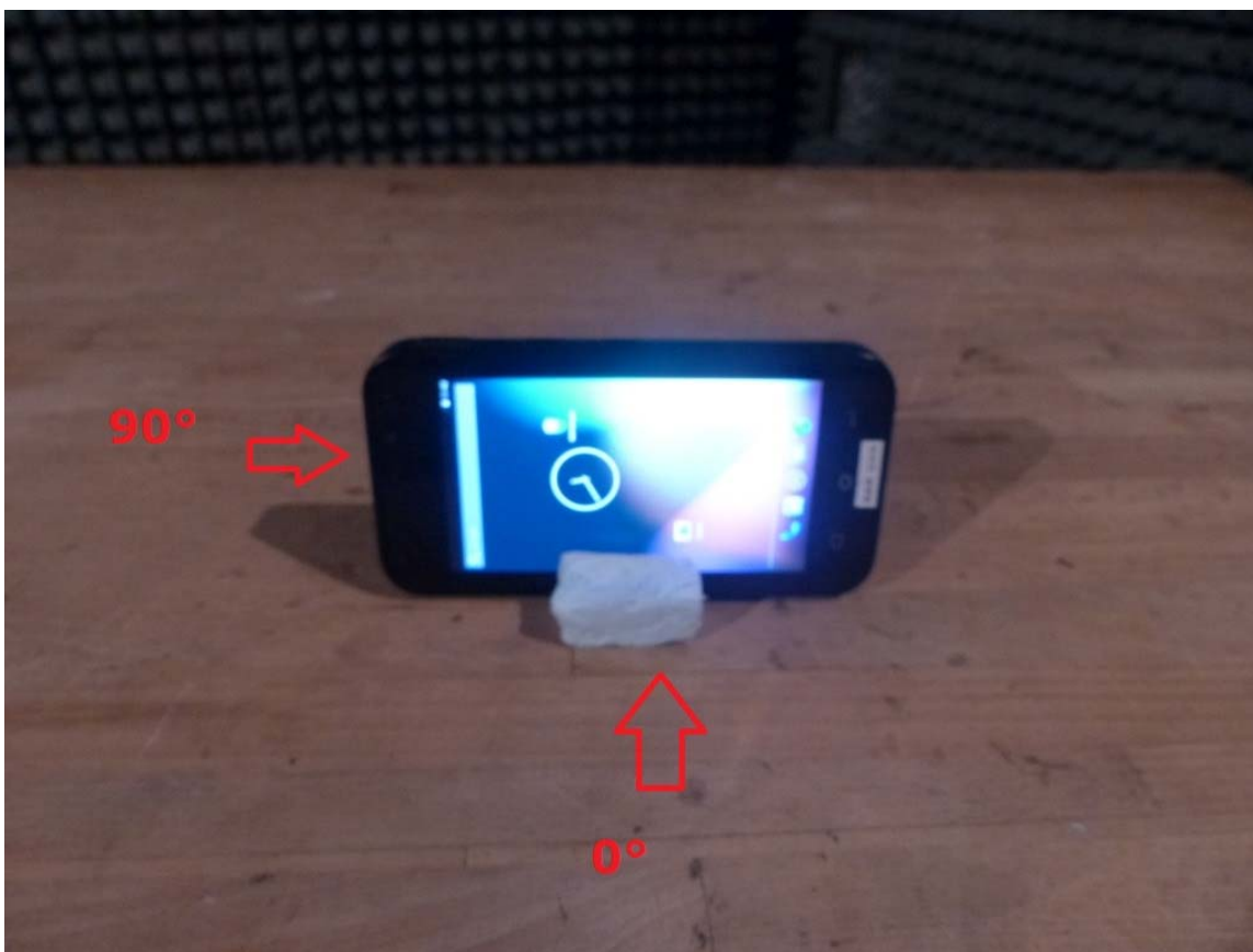
Photo 1: Equipment under test and definition of test sides for radiated measurements
