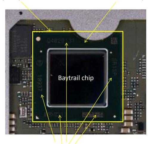
Processor markings are located on substrate of chip
