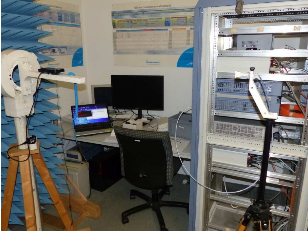
Photo 4: Test setup for radiated measurements (Enclosure, Outside of the anechoic chamber, 26-40 GHz intentional radiator §15)
