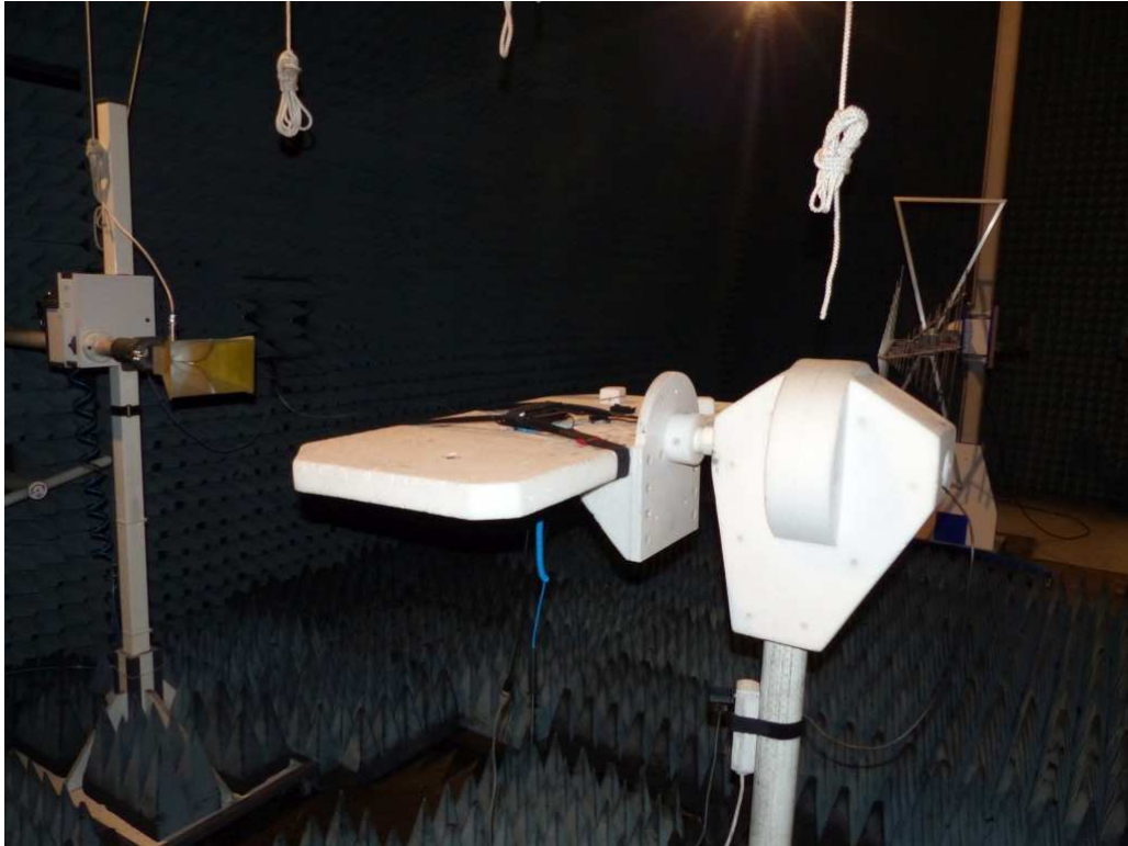
Photo 3: Test setup for radiated measurements (Enclosure, fully-anechoic chamber, 1-26 GHz intentional radiator §15)
