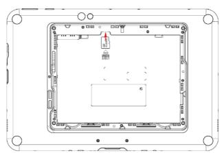
When putting the battery back in place, please make sure both hooks have clicked and are safely secured. Ensure to put the battery lid in place securely.
