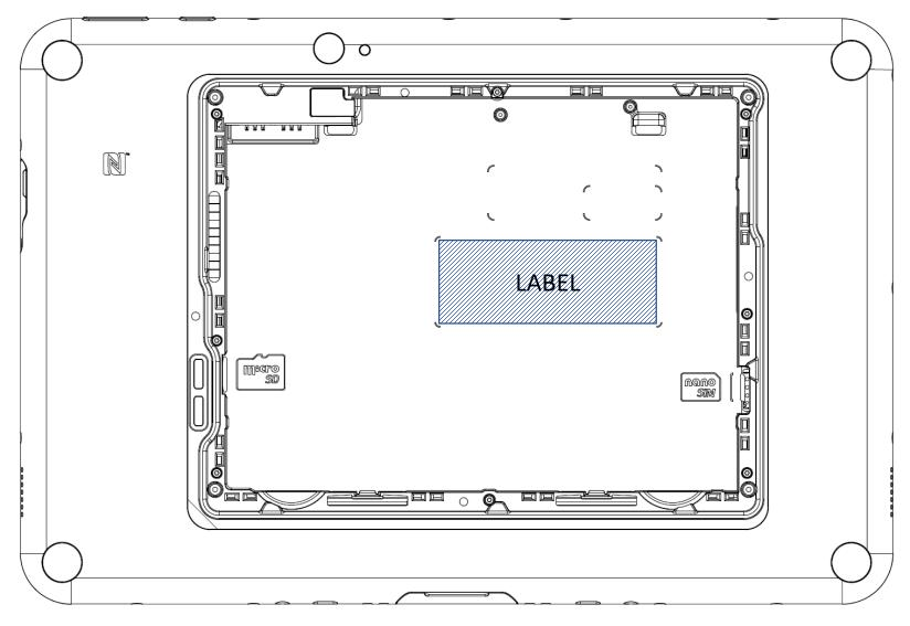
The label will be put inside the battery compartment. The label is visible to the users as they purchase the product and install the battery.
