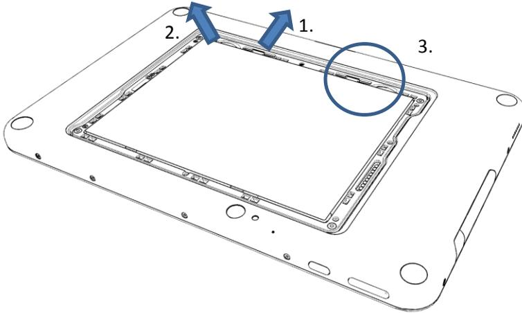
Enter the SIM card into the slot in the bottom right corner. Please make sure you have the SIM card in the correct direction (chip facing down).
