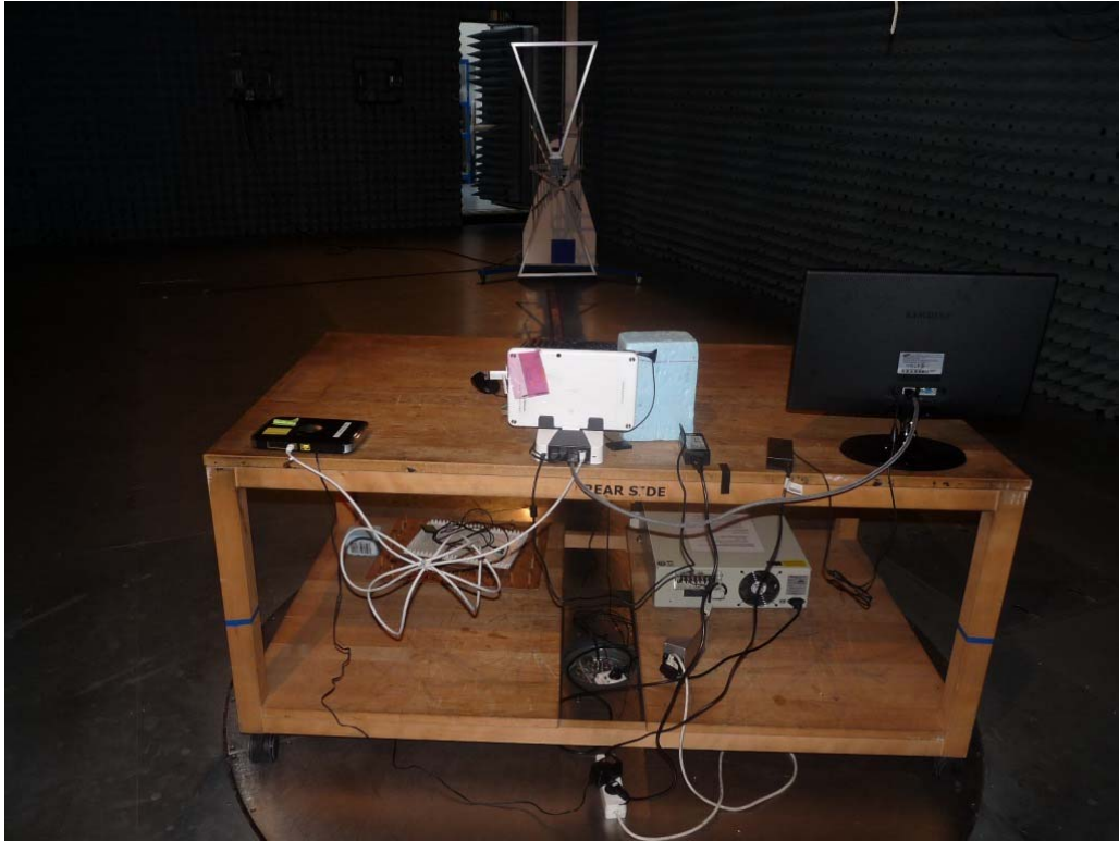
Photo 4: Test setup for radiated measurements (computer peripheral setup, EUT supplied by battery, unintentional radiator §15)
