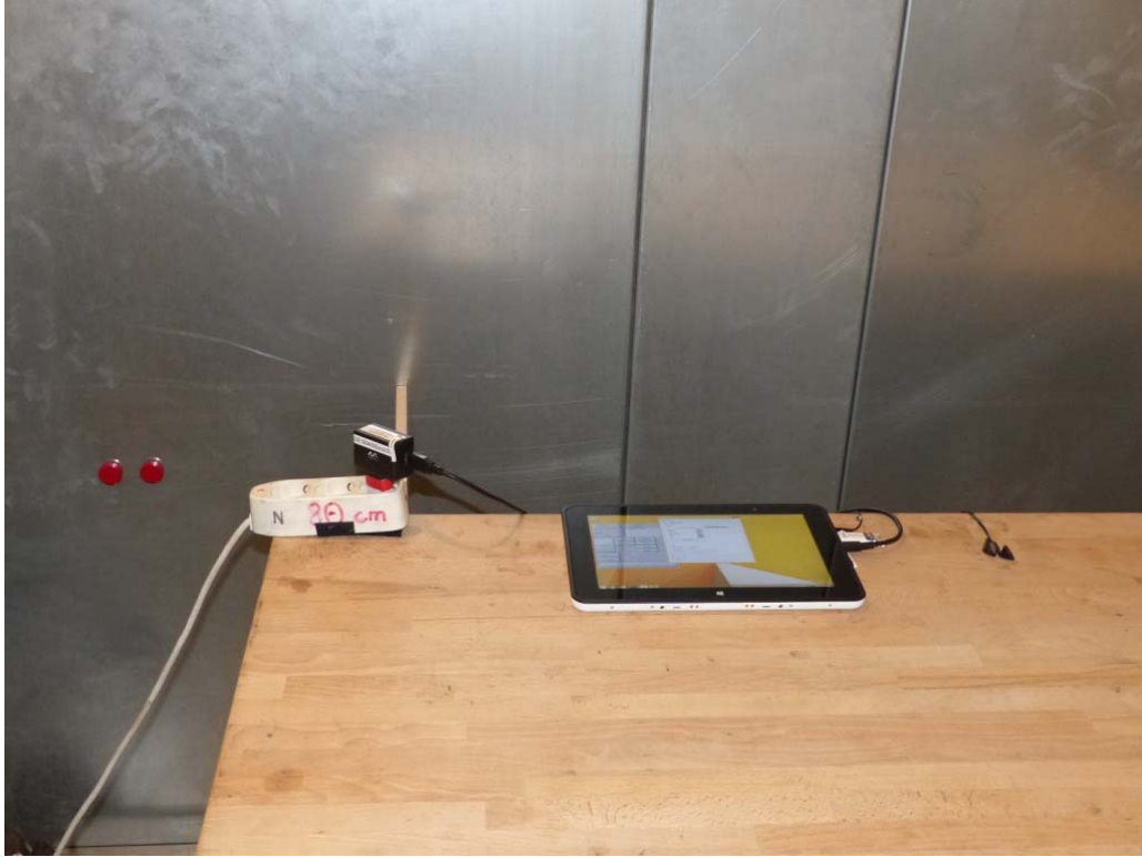
Photo 1: Test setup for conducted measurements (AC Port (power line), EUT supplied by battery, intentional / unintentional radiator §15)
