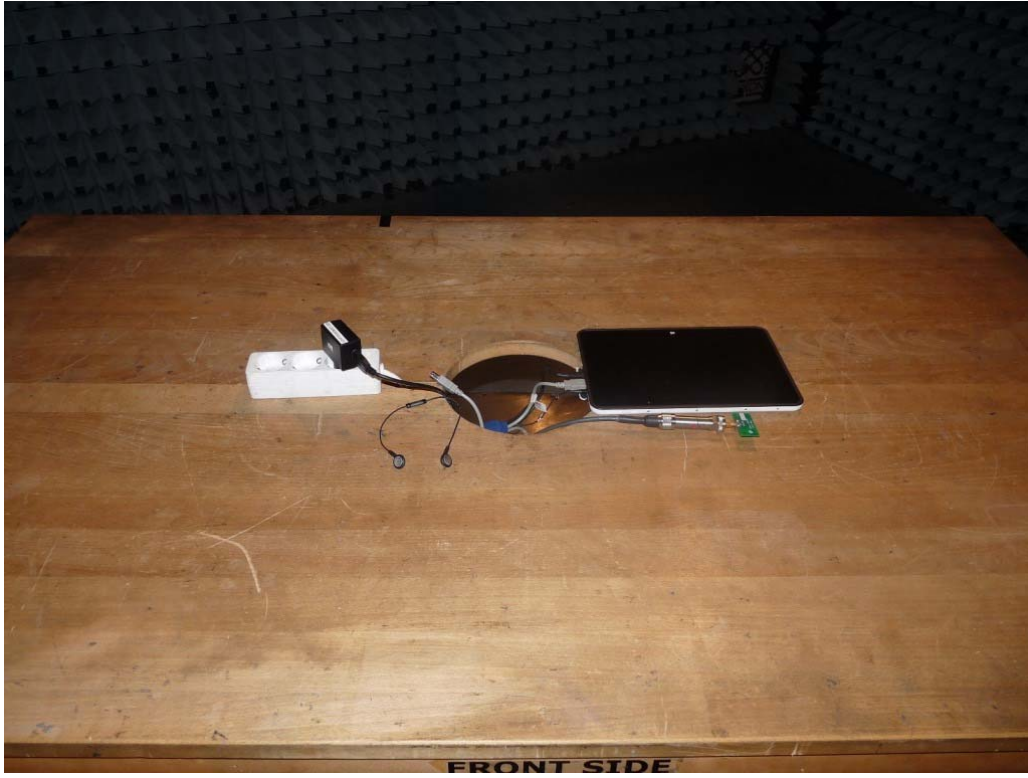
Photo 3: Test setup for radiated measurements (AC Port (power line), EUT supplied by battery, unintentional radiator S15)
