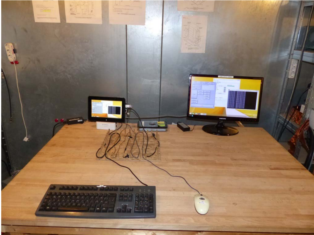
Photo 2: Test setup for conducted measurements (computer peripheral setup, EUT supplied by battery, unintentional radiator §15)
