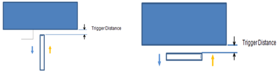
Picture: Proximity sensor triggering distance assessment Top side and Left side
