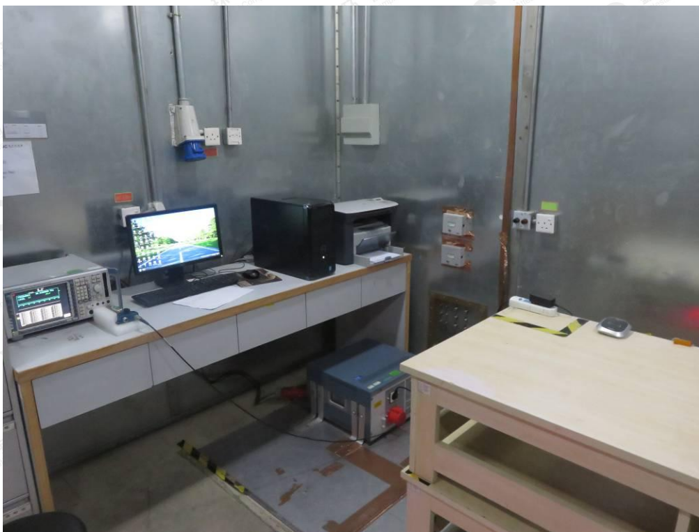
FCC RADIATED EMISSION TEST SETUP
