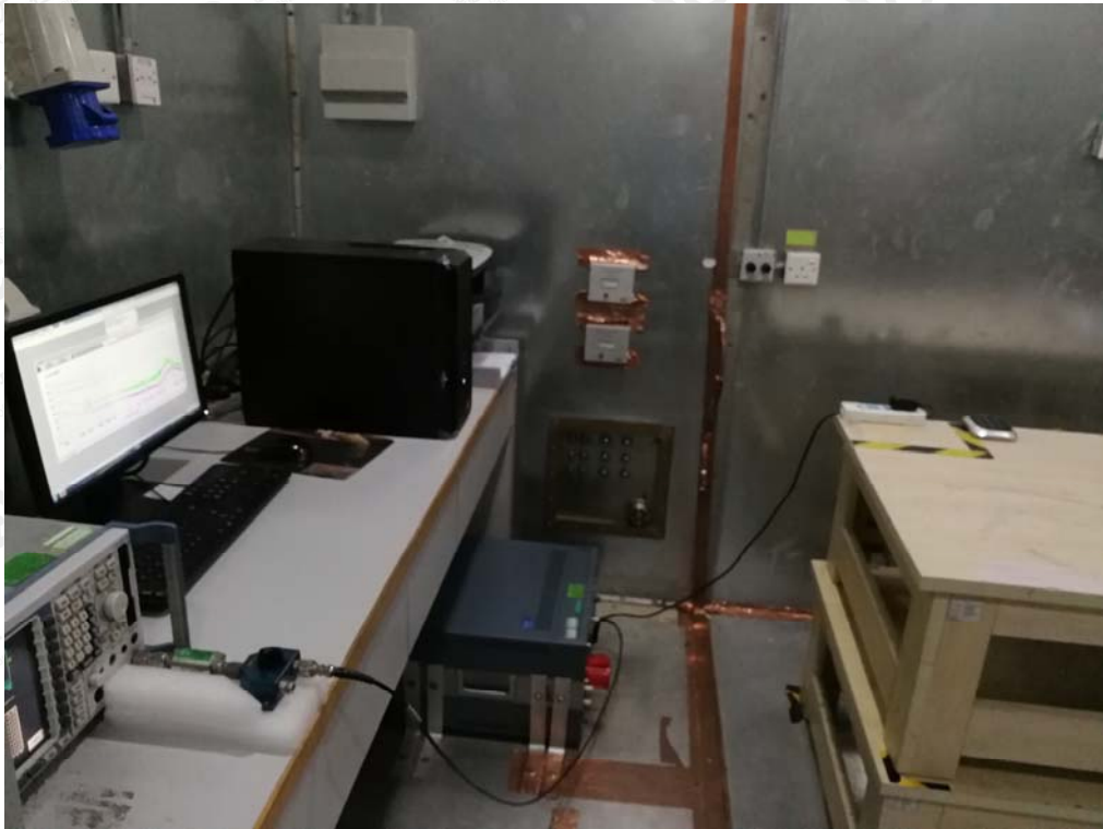
RADIATED EMISSION TEST SETUP BELOW 30MHz
