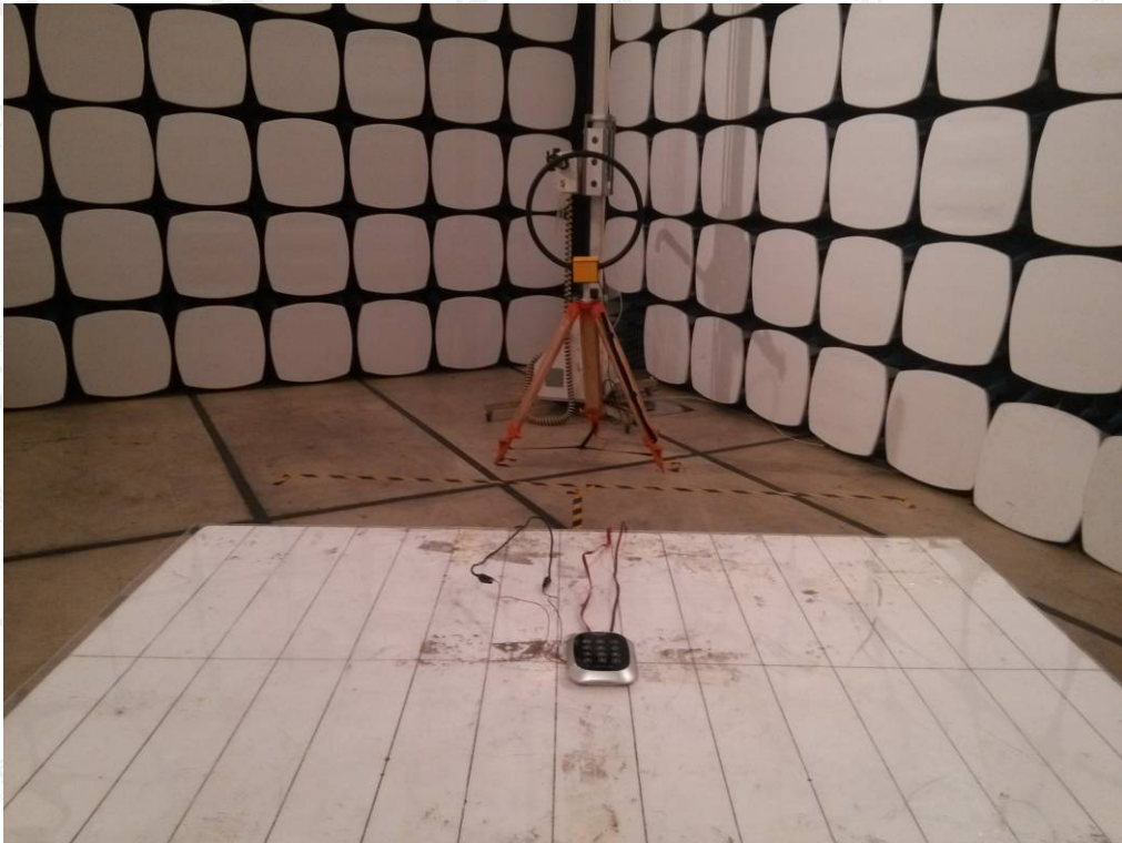
RADIATED EMISSION TEST SETUP BELOW 30MHz
