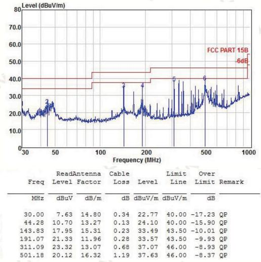
Remark: Absolute Level = Reading Level + Factor, Margin = Absolute Level – Limit Factor = Ant. Factor + Cable Loss – Pre-amplifier
