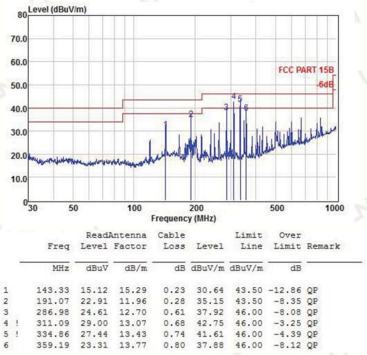
Remark: Absolute Level = Reading Level + Factor, Margin = Absolute Level – Limit Factor = Ant. Factor + Cable Loss – Pre-amplifier
