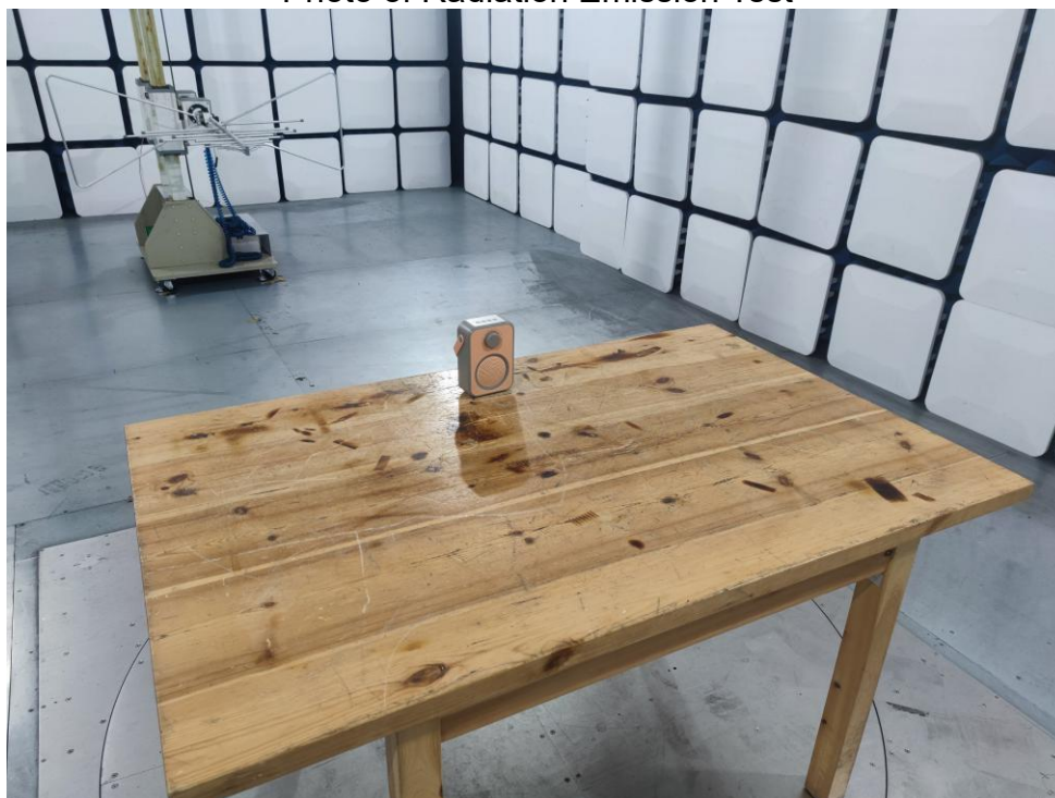
Photo of Radiation Emission Test
