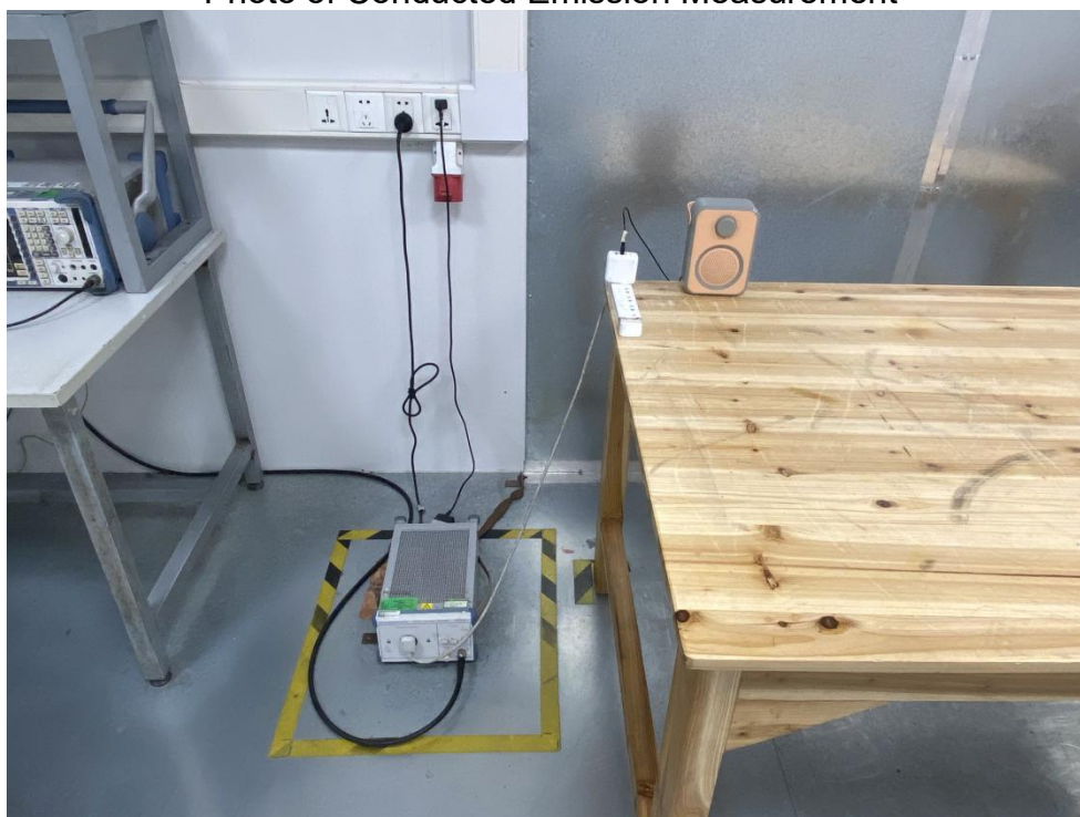
FCC ID:2ABV4PBT9550 Photo of Conducted Emission Measurement
