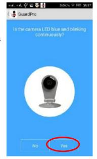
Insert a pin into the reset button on the back of the camera, press down and hold for 5 seconds. Wait for the camera to reset and the blue light to blink.
