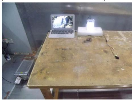
2 Photograph – Radiated Emission Test Setup for 30~1000MHz at Test Site 2#
