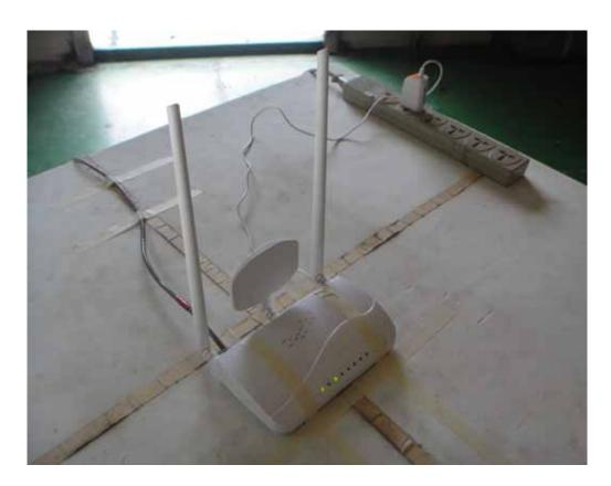
ANTENNA PORT CONDUCTED RF MEASUREMENT SETUP
