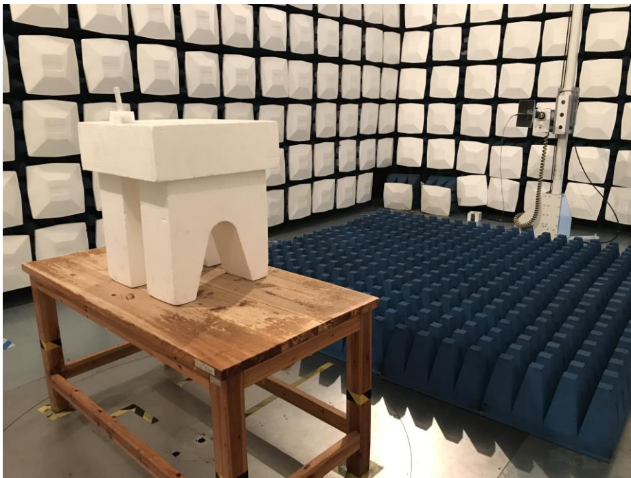
Test Setup For Radiated Emission (Above 1GHz)
