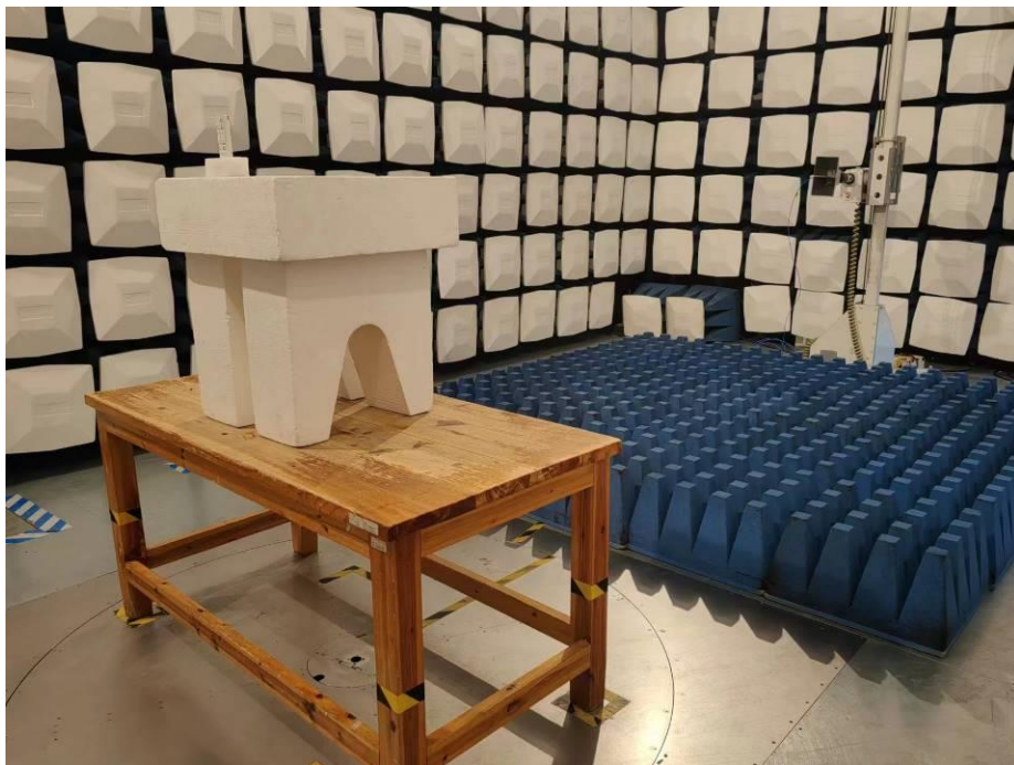
Test Setup For Radiated Emission (Above 1GHz)
