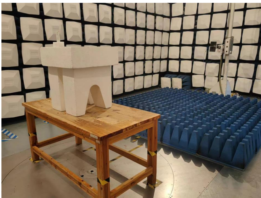
Test Setup For Radiated Emission (Above 1GHz)
