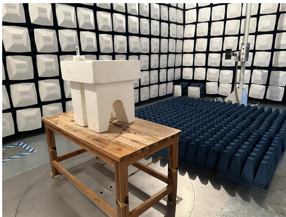
Test Setup For Radiated Emission (Above 1GHz)
