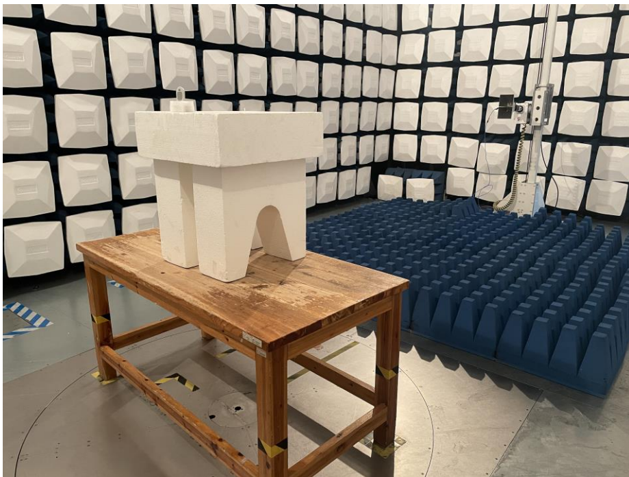
Test Setup For Radiated Emission (Above 1GHz)
