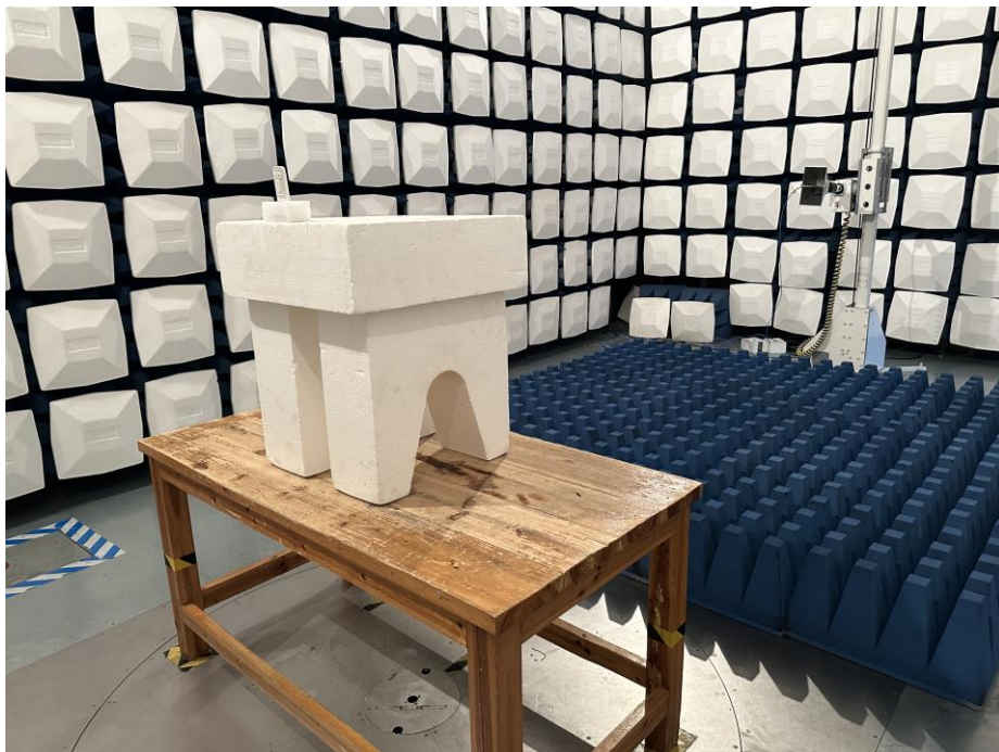
Test Setup For Radiated Emission (Above 1GHz)
