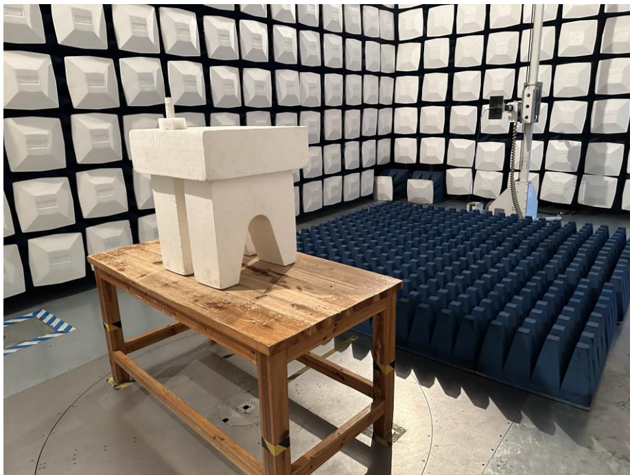
Test Setup For Radiated Emission (Above 1GHz)
