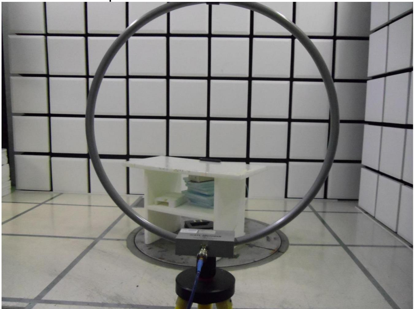
**Transmitter Radiated Spurious Emissions- 30 MHz-1 GHz**
