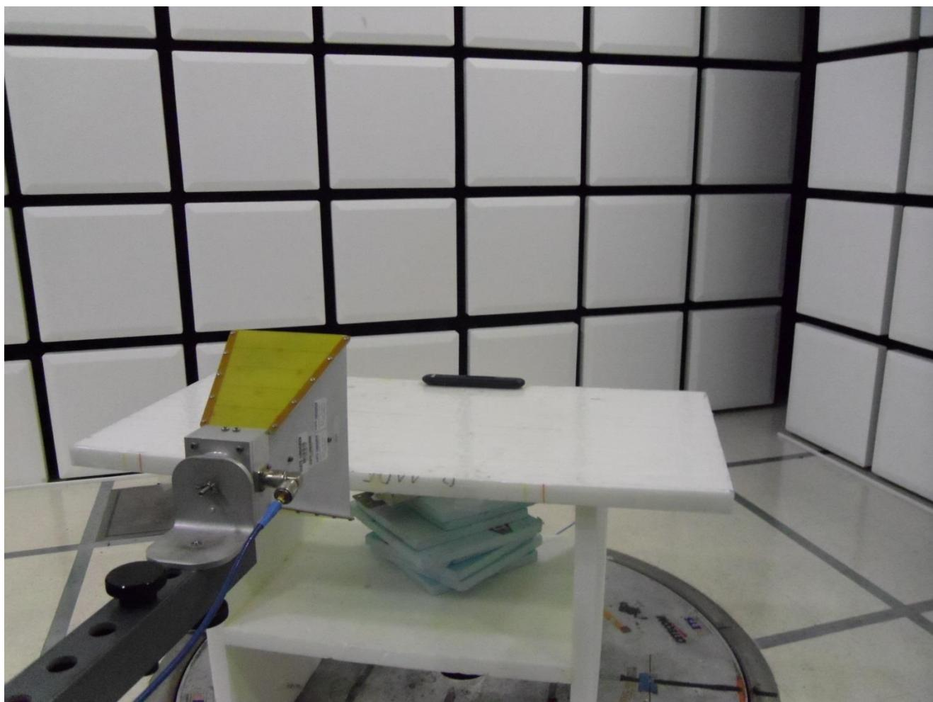
**Transmitter Radiated Spurious Emissions- 18-26 GHz**
