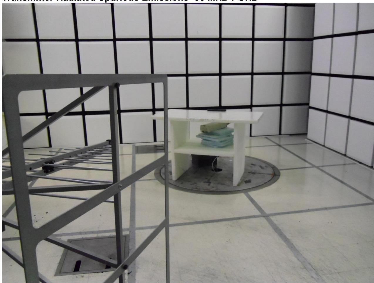
**Transmitter Radiated Spurious Emissions- 1-18 GHz**
