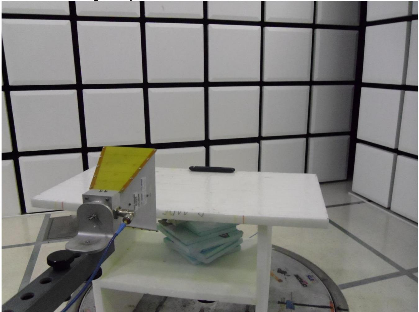
**Transmitter Radiated Spurious Emissions- 9 KHz-30 MHz**
