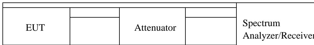
The EUT was directly connected to a RF Communication
