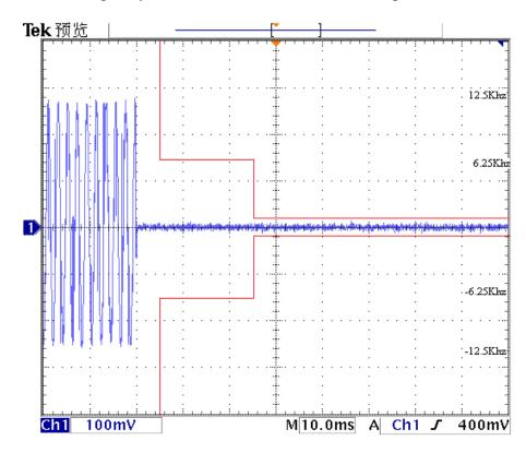
Transmitter Frequency Behavior @ 12.5 KHz Channel Separation-----On – Off
