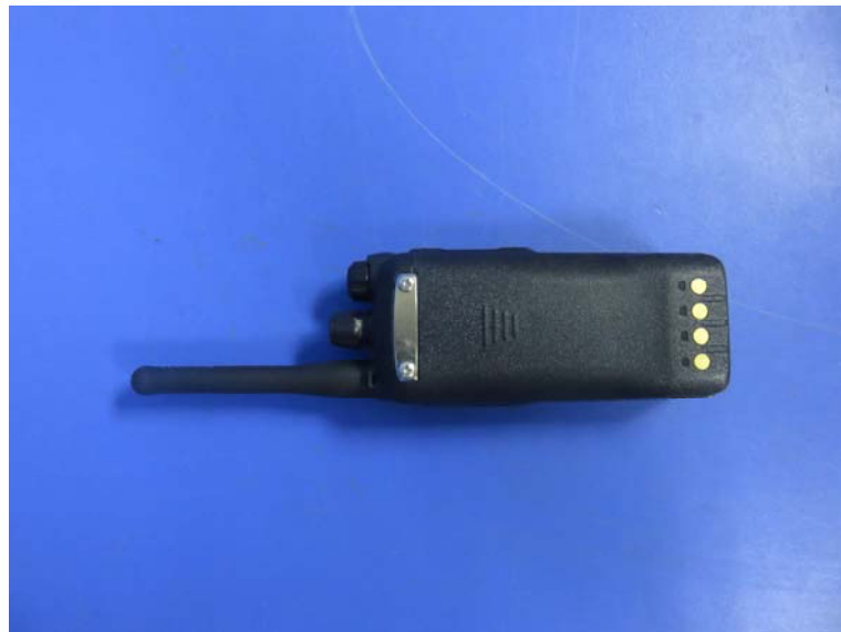
B1- Battery, Intrinsically Safe Li-ion Battery (B00237200)
