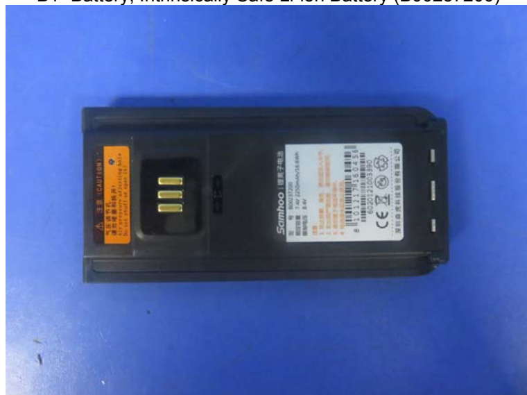
B1- Battery, Intrinsically Safe Li-ion Battery (B00237200)
