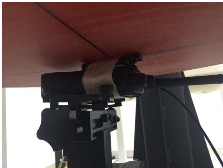
Body-worn, the front of the EUT towards ground with A1, B1, BC1 and AC3 (The distance was 0mm)
