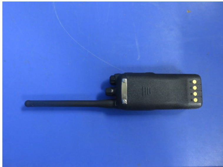
B1- Battery, Intrinsically Safe Li-ion Battery (B00237200)
