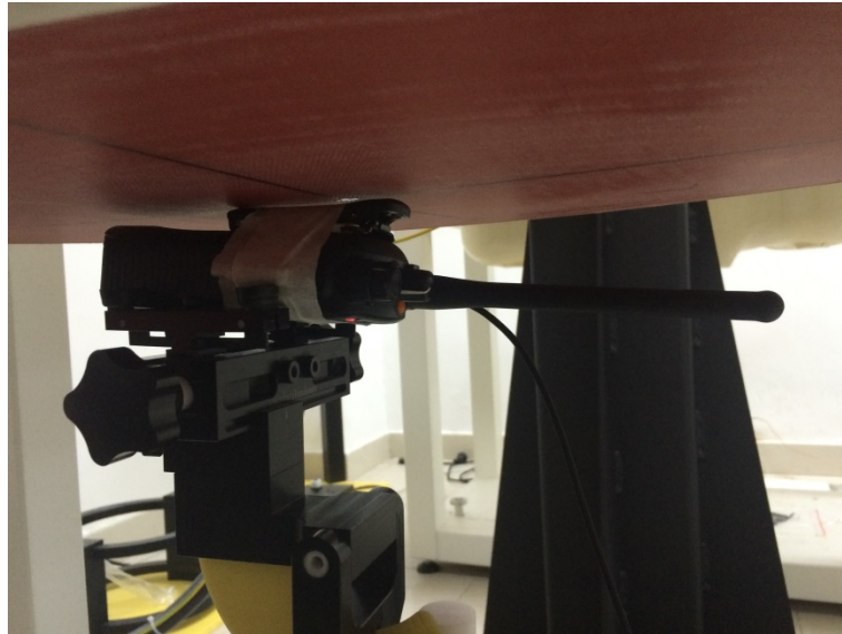
Body-worn, the front of the EUT towards ground with A1, B1, BC1 and AC2 (The distance was 0mm)
