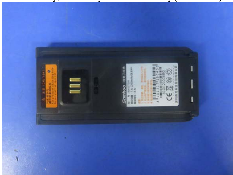
B1- Battery, Intrinsically Safe Li-ion Battery (B00237200)
