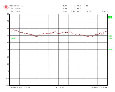
No frequencies were found inside the restricted bands during the preliminary radiated emission measurement.
