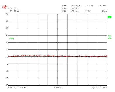
No significant emissions above the noise floor of the measuring system found, so no measurements on the outdoor test site were carried out.
