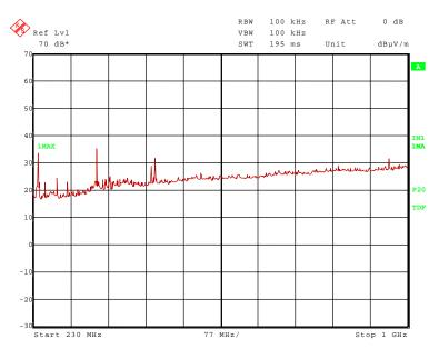
The following frequencies were found outside the restricted bands during the preliminary radiated emission measurement:
