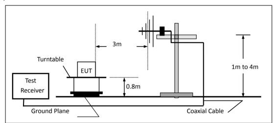
(c) For radiated emissions above 1000MHz
