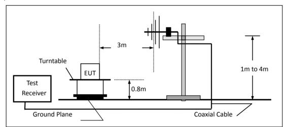
(c) For radiated emissions above 1000MHz
