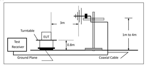
(c) For radiated emissions above 1000MHz
