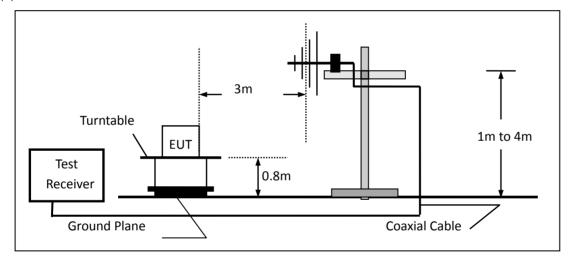
(c) For radiated emissions above 1000MHz
