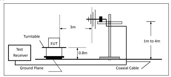
(c) For radiated emissions above 1000MHz
