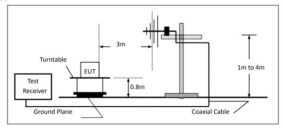
(c) For radiated emissions above 1000MHz
