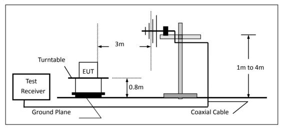
(c) For radiated emissions above 1000MHz
