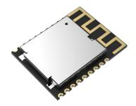
UART module MS48SF2 is based on m1805 Chipset. It is a small size (16×12×2mm) and stand-alone module with 12 GPIO. The data transmission between module and mobile phone can be achieved via operation of UART. With up to 60-meter working distance in open space, 512KB flash memory, etc., the data can be transmitted via Bluetooth
