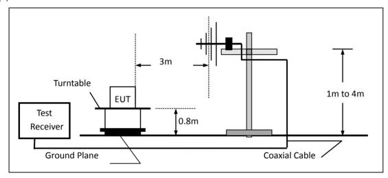
(c) For radiated emissions above 1000MHz
