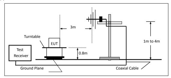
(c) For radiated emissions above 1000MHz
