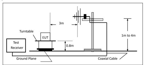
(c) For radiated emissions above 1000MHz
