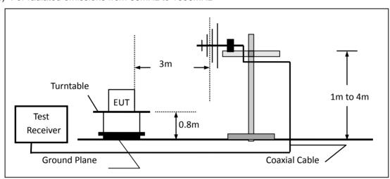
(c) For radiated emissions above 1000MHz
