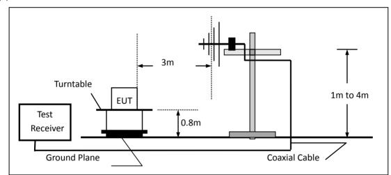
(c) For radiated emissions above 1000MHz
