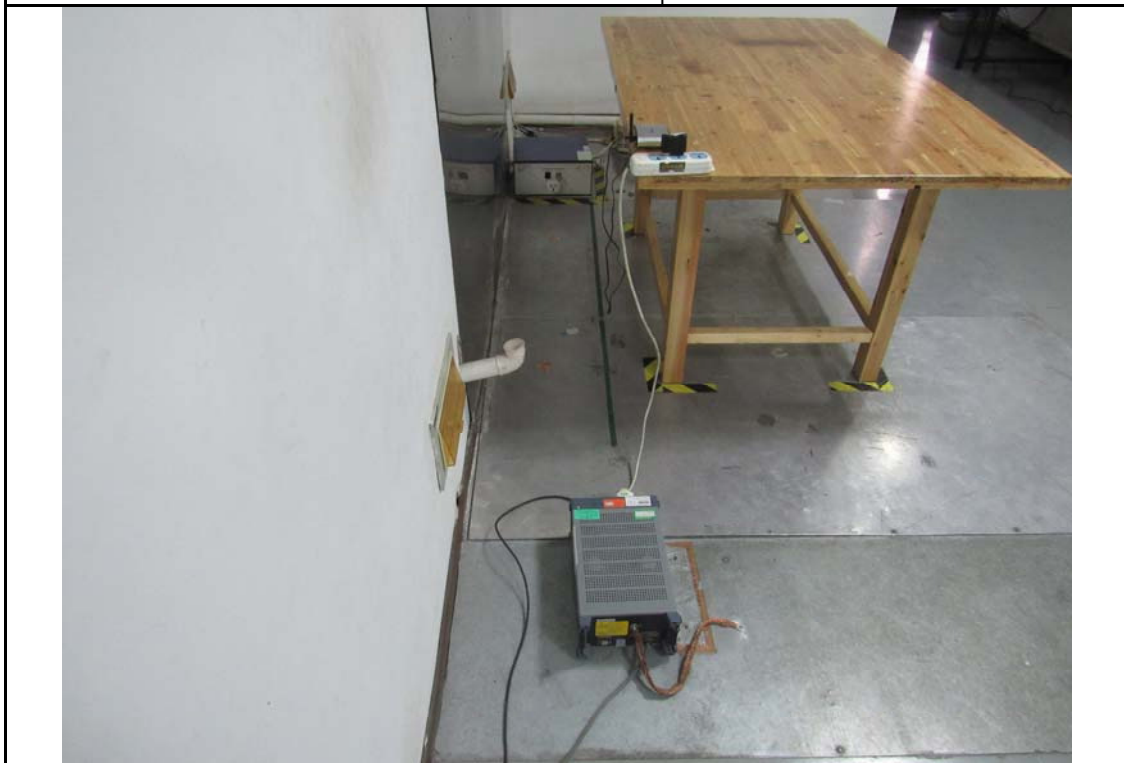
Conducted Emissions Test Setup Side View
