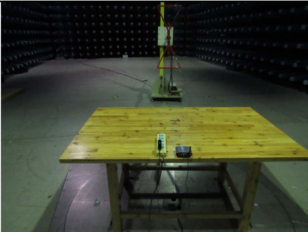
Radiated Spurious Emissions Test Setup Below 1GHz
