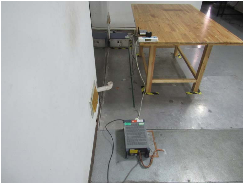
Conducted Emissions Setup Side View
