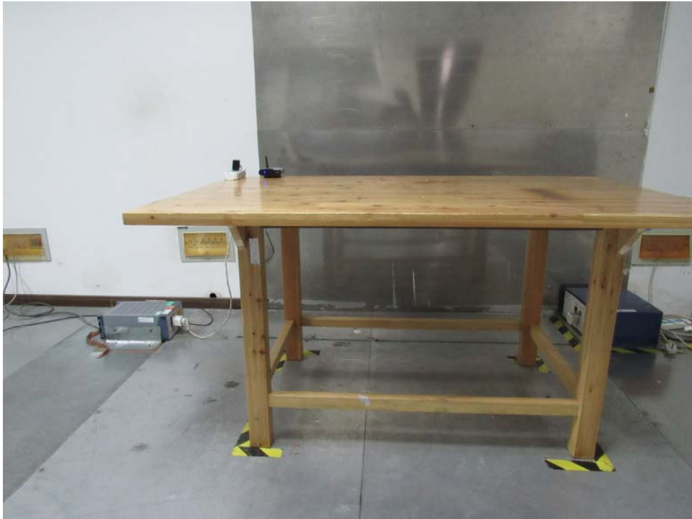
Conducted Emissions Setup Front View
