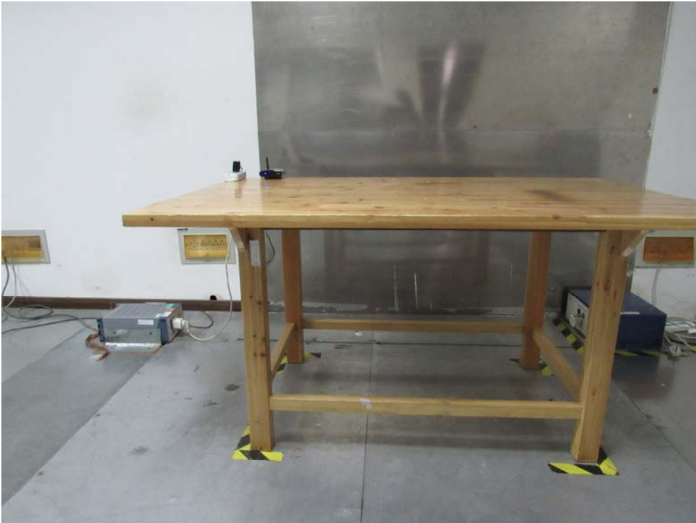
Conducted Emissions Setup Front View
