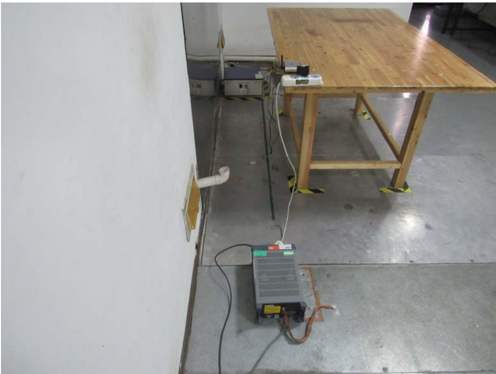
Conducted Emissions Setup Side View
