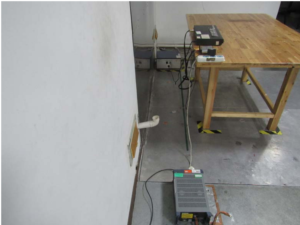
Conducted Emissions Setup Side View
