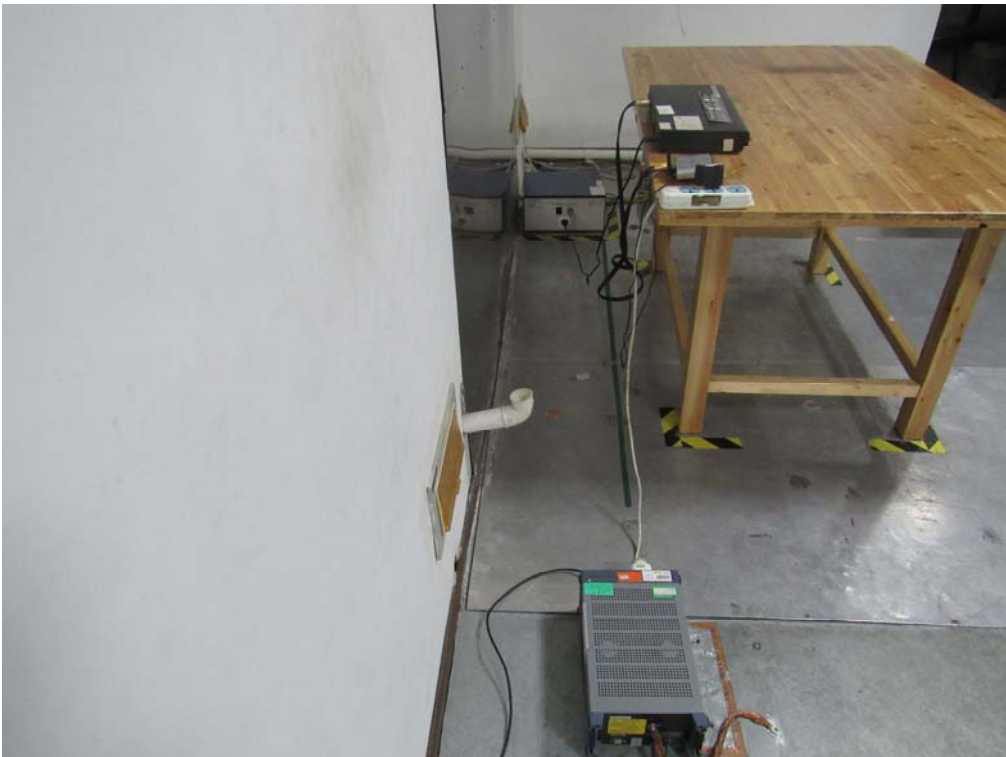
Conducted Emissions Setup Side View
