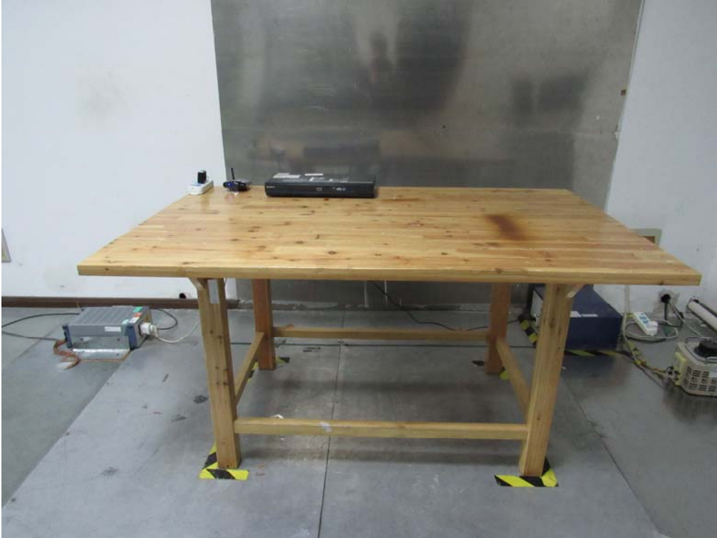
Conducted Emissions Setup Front View
