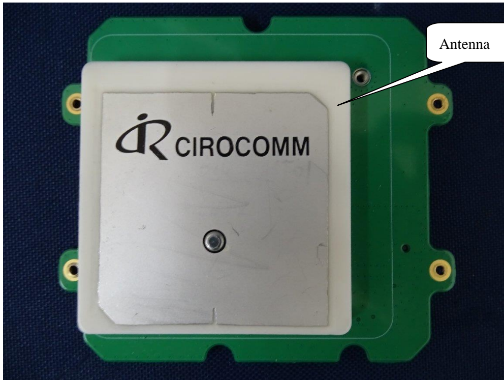
(2) EUT Photo-All PCB is a Module
