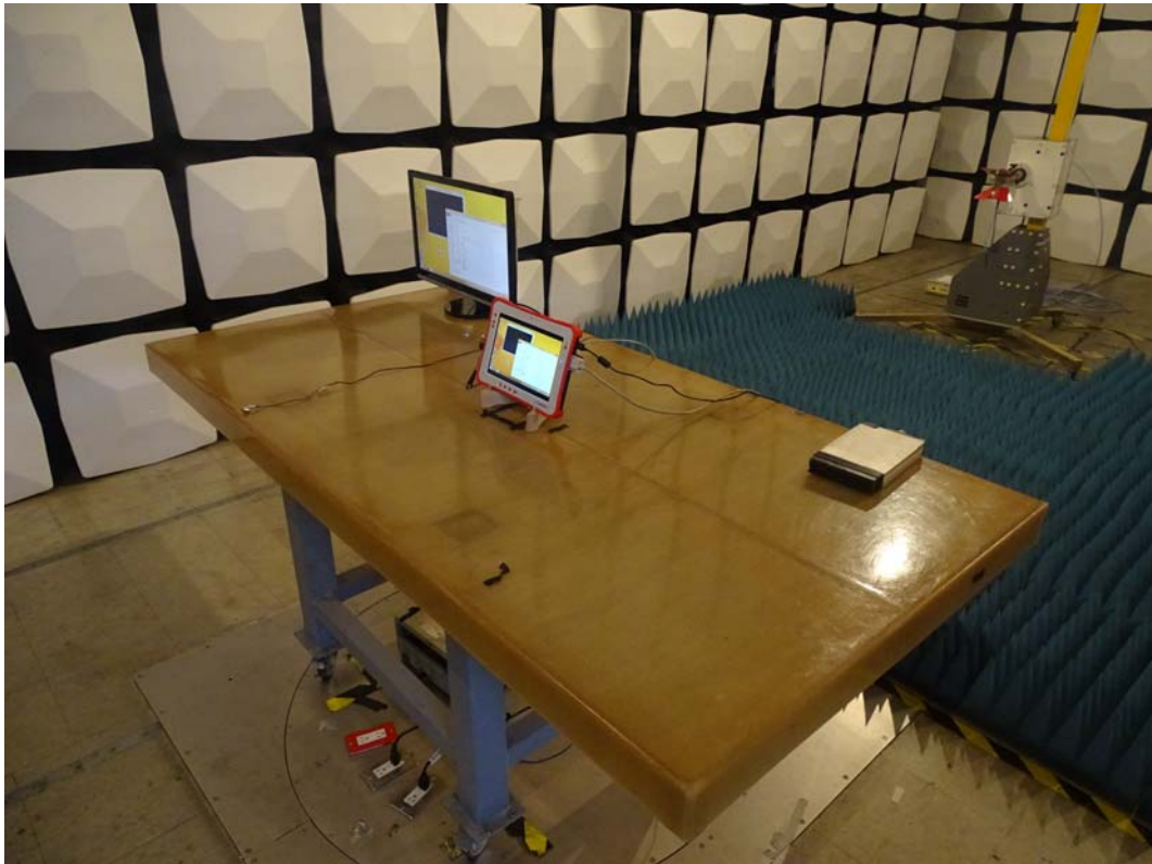
Front View of Radiated Test
