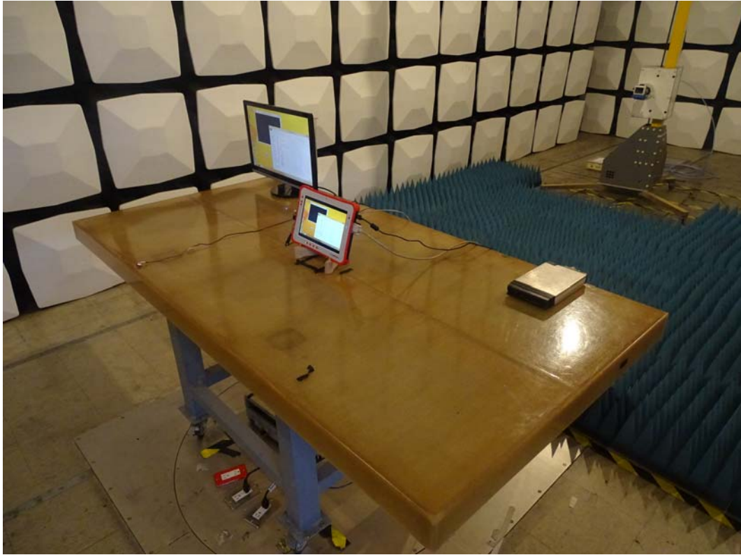
Front View of Radiated Test (Horn)
